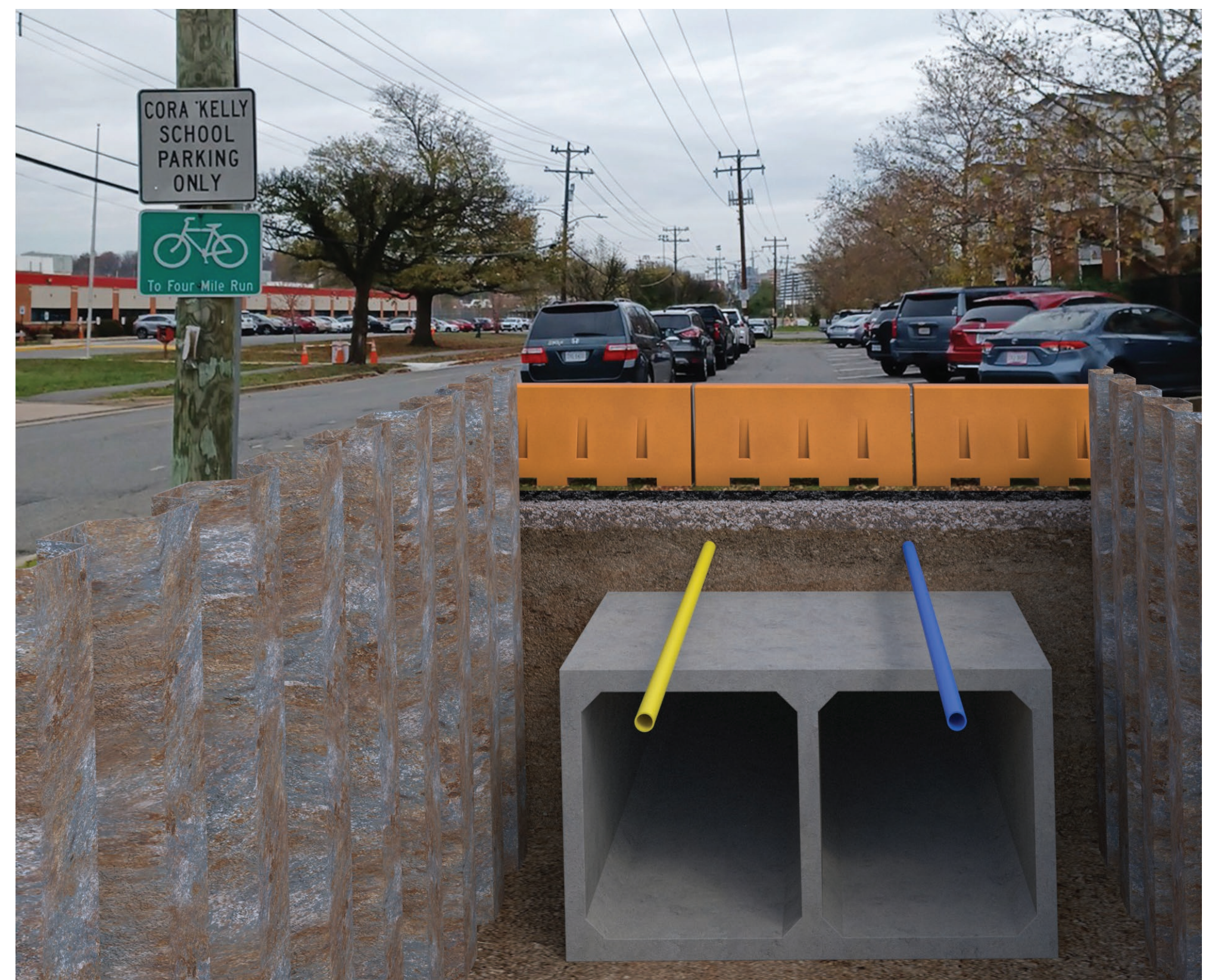
Two 7' x 8' box culverts will be installed on the east side of Commonwealth Ave
